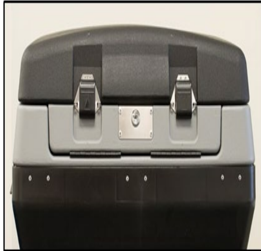
Figure - Unhooked Latches on Scanning Unit
