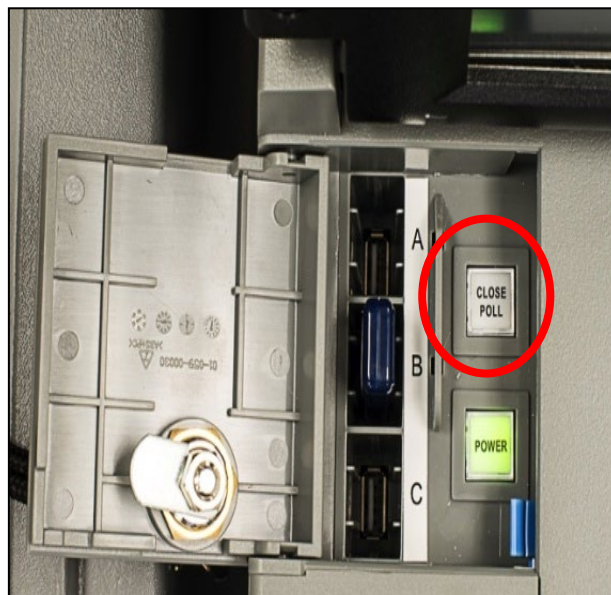
Figure - "Close Poll" Button in the Front Access Door
