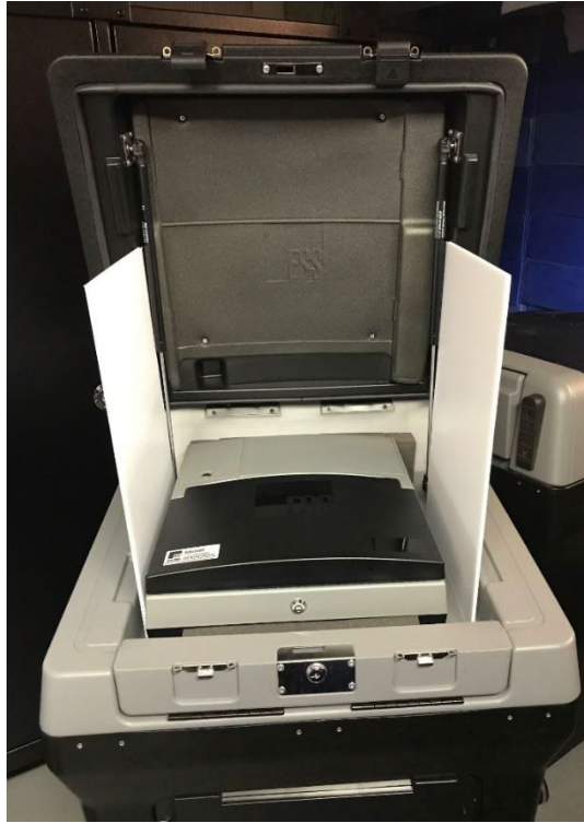
Figure - Privacy Screens on the Scanning Unit
